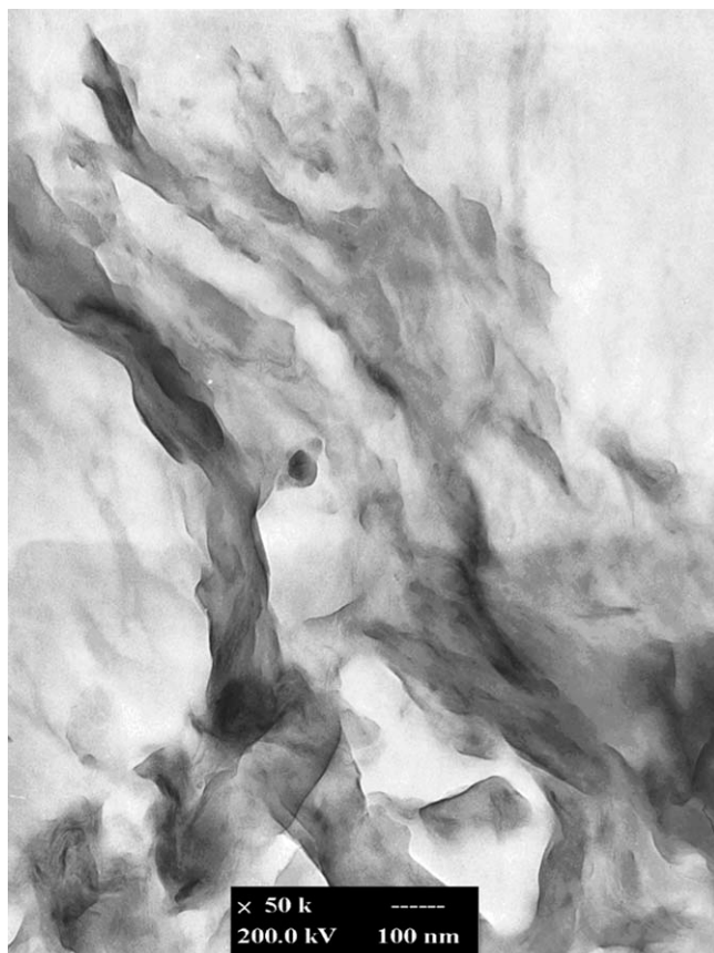
Figure 2 TEM micrograph ( \times 50,000 ) of the PLLA/ o -MMT nanocomposite incorporating 10 wt % MMT.
